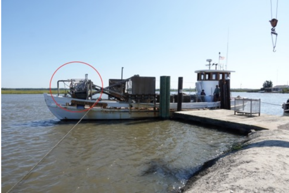
The oyster boat Peter Paynter prepares to off-load oysters by crane. The tumblers on the bow are culling machines. Photo September 2023: J. Morton Galetto
