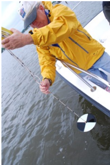
Water monitor Chesapeake Bay checks water quality with a Secchi disk. Photo: Chesapeake Bay Executive Order.
