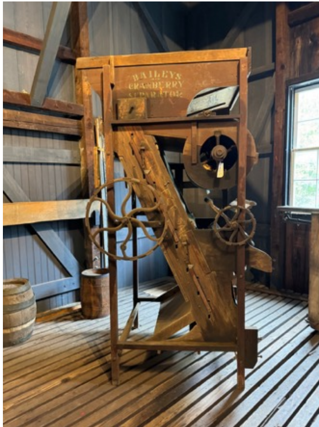
H.R. Baileys Cranberry Separator (patented 1923), is a machine which relied on "bounce" to sort berries, is exhibited at the Whitesbog Museum.
