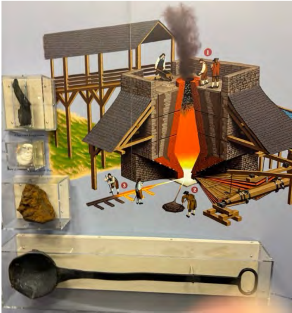
Iron ore was top loaded into a furnace c. 1820 to make iron bars called pigs. Molten material flowed into a main channel and then into side troughs resulting in a form resembling suckling pigs – thus pig iron. Display Batsto Village Visitor Center. Photo J. Morton Galetto
